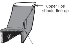
Cut away shows correct joint alignment
