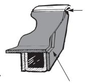
Cut away shows correct joint alignment
