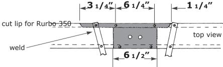
Install as shown in diagram. Weld in place with edge gaps to the front.
