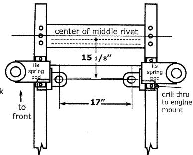
Bolt in place once mounts have been securely clamped. Drill 3/8 inch mounting holoes as shown above. Use 4 bolts per side, one each on top and bottom plus two into each IFS pod.
