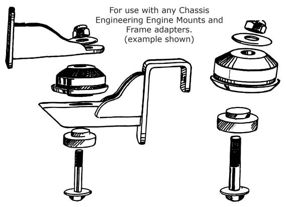
See the catalog or go to the Engine Mount Kit section on www. chassisengineeringinc.com for selecting the correct frame adapter and engine mount. Engine mounts are available for Ford and Chevy Small Block, Chevy 6cyl, Chrysler V8 (including early HEMI) and others.
