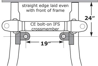
Bolt engine mounts to block and install engine. Installer is responsible for final fit. Generally the frame mounts will clear the IFS with no problems. Make sure to install the cushion set as shown.
