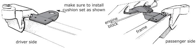
Note: engine mounts are both the same and both offset. This makes both sides equal when installed.
