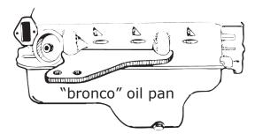
The original oil pan can be notched for clearance as well.
