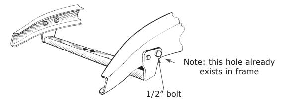
2 Level mount and drill smaller holes thru frame.
