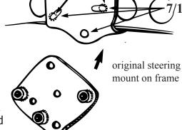
The drag link will need to be shortened about 3/4". This can usually be done by using the adjustment already there. The gearbox should be in the exact center position with wheels pointed straight ahead. This is important!
